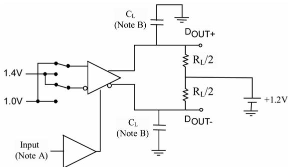
Note A: All LVTTTL input pulses have frequency = 10MHz,  $t_R$  or  $t_F \le 2\text{ ns}$
