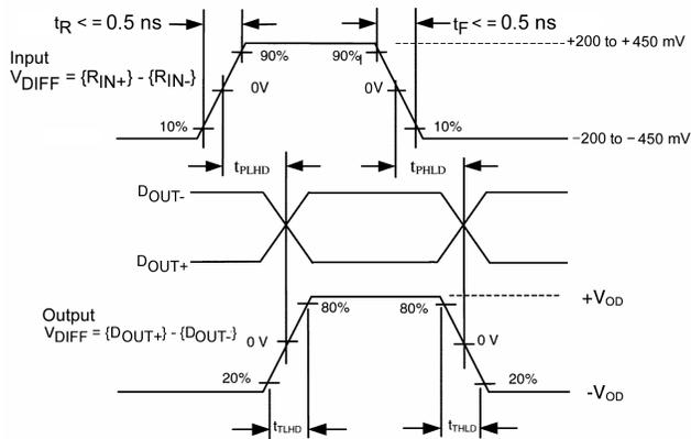
FIGURE 4. AC Waveform
