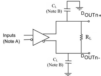
**Note A:** All LVDS input pulses have frequency = 10 MHz,  $t_R$  or  $t_F < 0.5 \text{ ns}$
