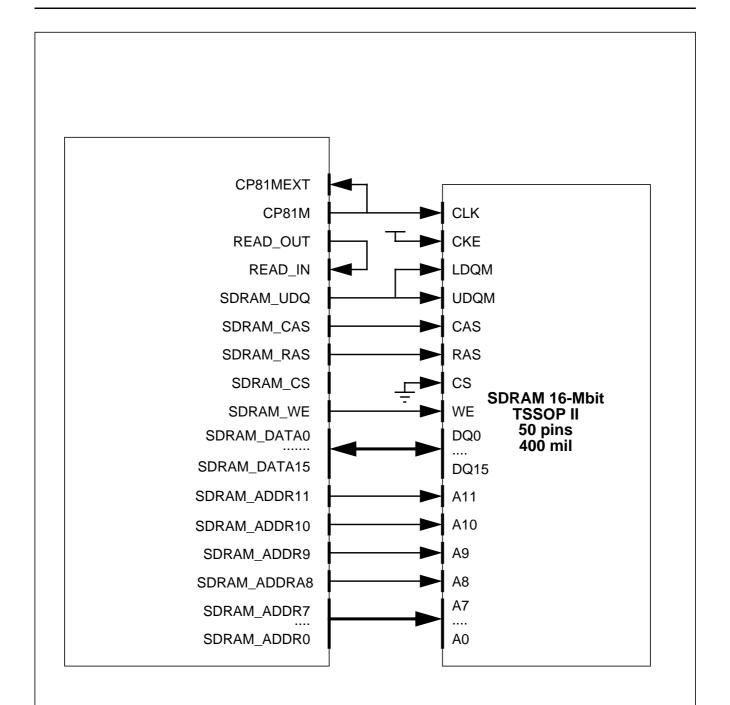
The board should be designed to insure a similar load on the CP81M and READ\_OUT pins as well as a similar fly time between the CP81M and CP81MEXT pins on one side and the READ\_OUT and READ\_IN pins on the other side.
