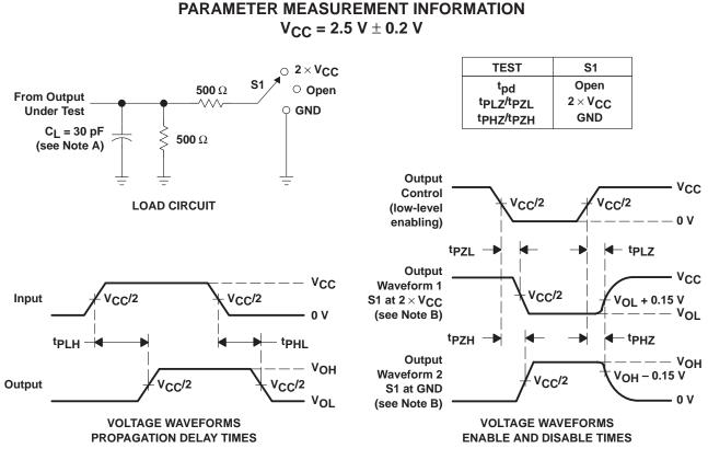
NOTES: A. CL includes probe and jig capacitance.
