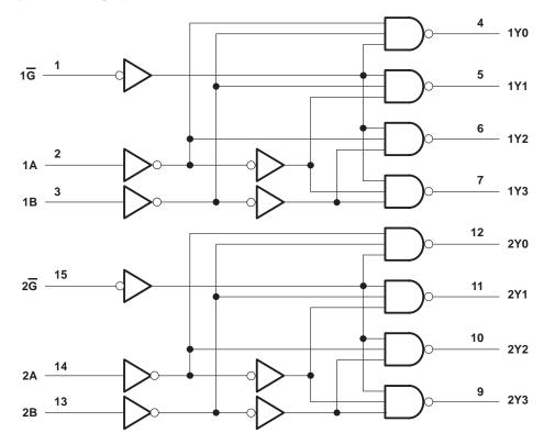
Pin numbers shown are for the D, DB, DGV, J, NS, PW, and W packages.
