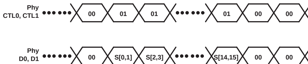
Figure 6. Status Transfer Timing
