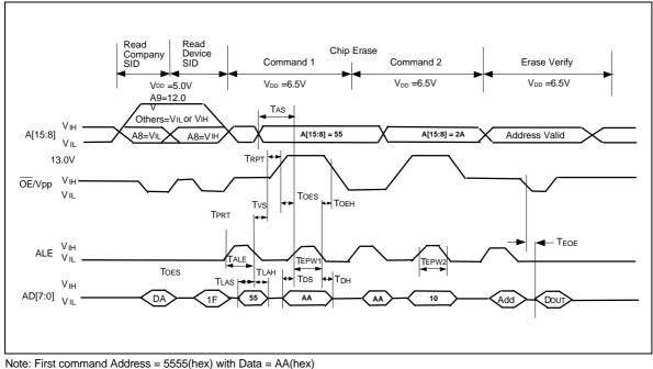
Second command Address = 5555(nex) with Data = AA(nex) Second command Address = 2AAA(hex) with Data = 10(hex)
