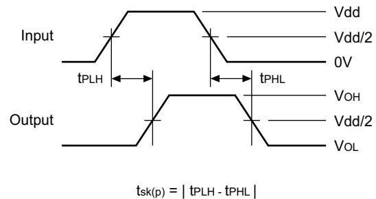
$$t_{SK(P)} = | t_{PLH} - t_{PHL} |$$
