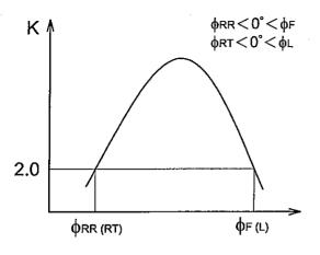
Contrast ratio K vs viewing angle φ
