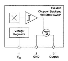
The FUS5881 Hall-Effect sensor IC family is designed in CMOS technology providing chopper stabilized amplifiers with switched capacitors. Therefore these magnetic field sensor devices have no amplifier offset voltage which in bipolar designed devices is the main reason for temperature sensitive output signal drift.
