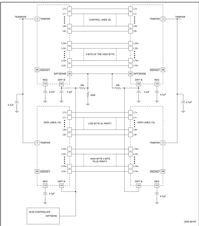
**Note:** A 220k resistor is added to ground to insure the transceivers will come up in single-ended mode when no terminator is enabled. The controller DIFFSENS ties to the DIFFB pin on the terminators, only one RC network should be on a device.
