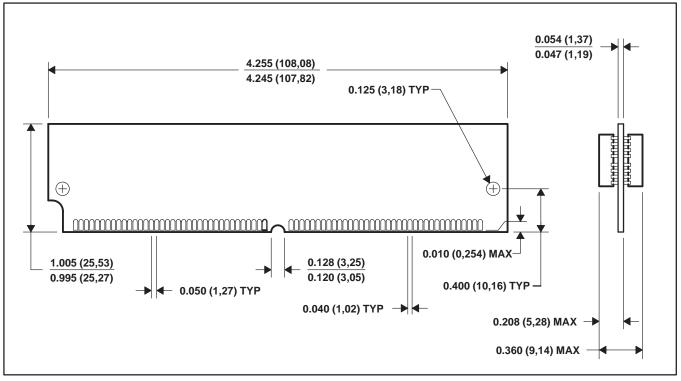
NOTE A: All linear dimensions are in inches (millimeters).
