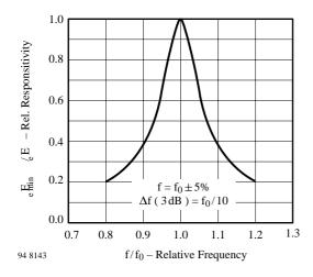
Figure 1. Frequency Dependence of Responsivity
