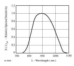
Figure 11. Relative Spectral Sensitivity vs. Wavelength
