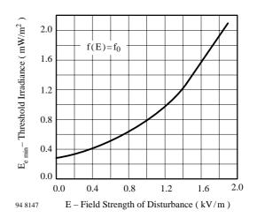
Figure 4. Sensitivity vs. Electric Field Disturbances
