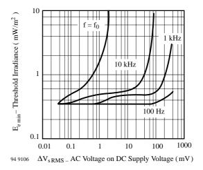
Figure 5. Sensitivity vs. Supply Voltage Disturbances
