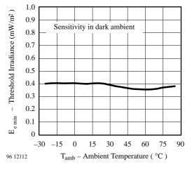
Figure 6. Sensitivity vs. Ambient Temperature
