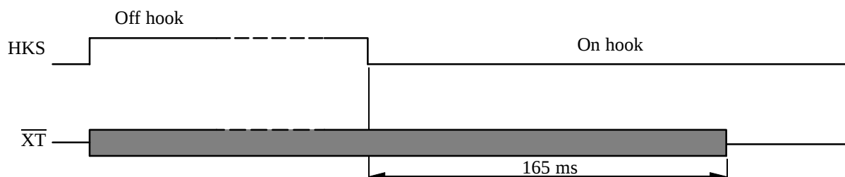
Figure 14. Symbolic timing diagram: on hook debounce time
