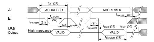
u:  $\overline{W}$  must be HIGH when  $\overline{E}$  is LOW during the address sequence in order to initiate a nonvolatile cycle.  $\overline{G}$  may be either HIGH or LOW throughout. Addresses 1 through 6 are found in the mode selection table. Address 6 determines whether the U635H64 performs a STORE or RECALL.
