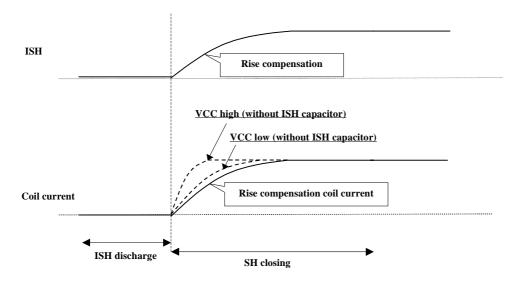
Setting the input voltage of ISH pin larger than the coil time constant by means of an external CR enables application of rise compensation to the coil waveform, ensuring stable shutter operation against fluctuation of power supply.
