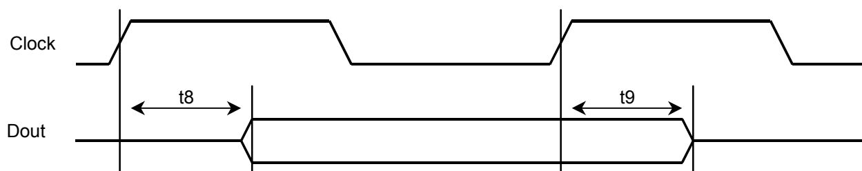
Figure 18-5. To/From High-Z Delay Definitions (Rising Clock Edge)
