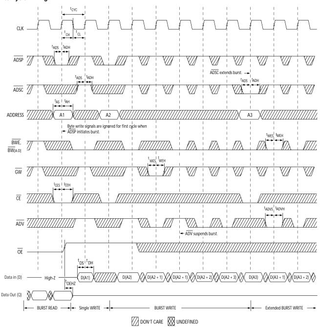
**Note:** 17. Full width write can be initiated by either  $\overline{GW}$  LOW; or by  $\overline{GW}$  HIGH,  $\overline{BWE}$  LOW and  $\overline{BW}_{[A:D]}$  LOW.
