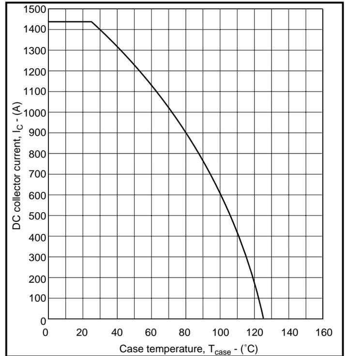
Fig. 12 DC current rating vs case temperature
