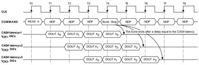
Termination of a Burst Read Operation (Burst Length > 4, CAS# Latency = 1, 2, 3)
