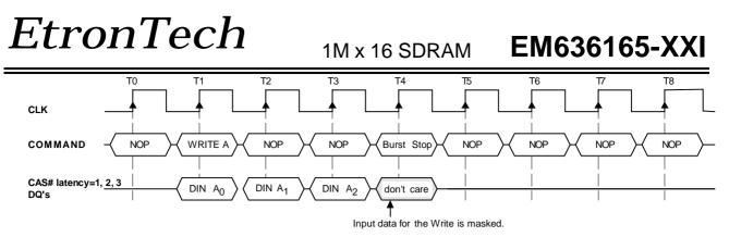
**Termination of a Burst Write Operation** (Burst Length = X, CAS# Latency = 1, 2, 3)
