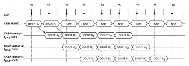
Read Interrupted by a Read (Burst Length = 4, CAS# Latency = 1, 2, 3)
