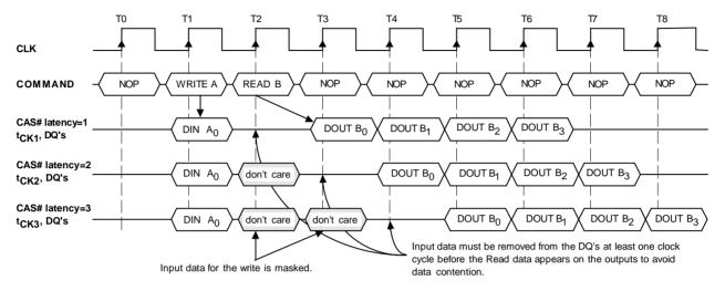
Write Interrupted by a Read (Burst Length = 4, CAS# Latency = 1, 2, 3)
