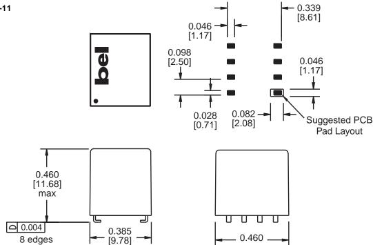
Dimensions are in inches [millimeters]. Standard dimension tolerance is ±0.005 [0.13] unless otherwise noted.
