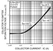
Fig.2 Collector-emitter saturation voltage vs. collector current
