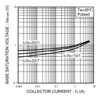
Fig.3 Base-emitter saturation voltage vs.collector current
