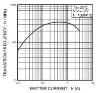
Fig.5 Gain bandwidth product vs. emitter current
