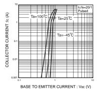
Fig.4 Grounded emitter propagation characteristics
