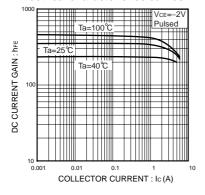
Fig.1 DC current gain vs. collector current
