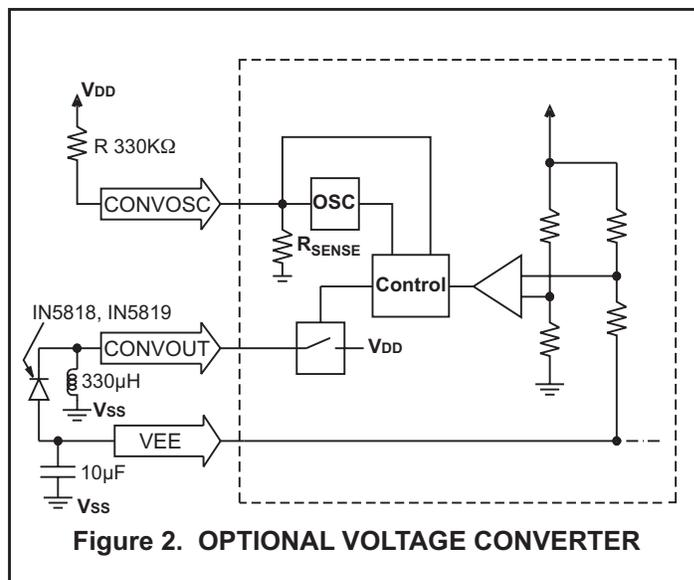
Figure 2. OPTIONAL VOLTAGE CONVERTER
