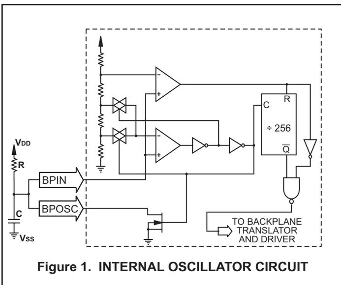
Figure 1. INTERNAL OSCILLATOR CIRCUIT
