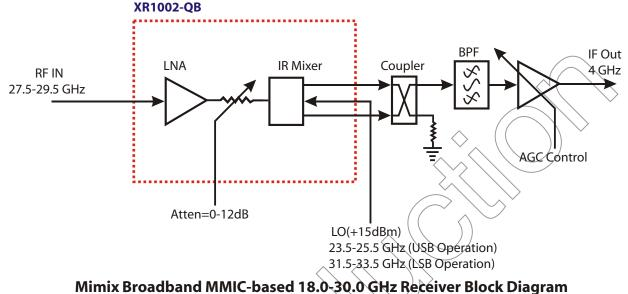
(Changing LO and IF frequencies as required allows design to operate as high as 30 GHz)
