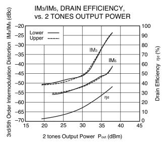
W-CDMA 3GPP, Test Model 1, 64 DPCH, 67% Clipping, Center Frequency 2.14GHz, 15 MHz spacing
