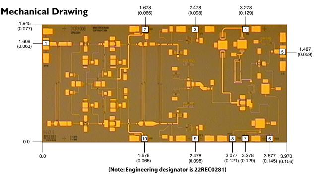
Units: millimeters (inches) Bond pad dimensions are shown to center of bond pad. Thickness: 0.110 +/- 0.010 (0.0043 +/- 0.0004), Backside is ground, Bond Pad/Backside Metallization: Gold All DC/IF Bond Pads are 0.100 x 0.100 (0.004 x 0.004). All RF Bond Pads are 0.100 x 0.200 (0.004 x 0.008) Bond pad centers are approximately 0.109 (0.004) from the edge of the chip. Dicing tolerance: +/- 0.005 (+/- 0.0002). Approximate weight: 4.787 mg.
