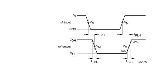
For 74HC3G:  $V_M$  = 50%;  $V_I$  = GND to  $V_{CC}$ . For 74HCT3G:  $V_M$  = 1.3 V;  $V_I$  = GND to 3.0 V.
