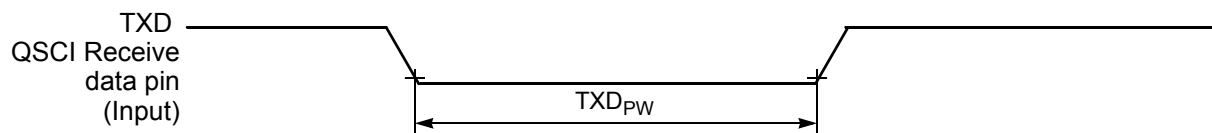
Figure 10-13 TXD Pulse Width
