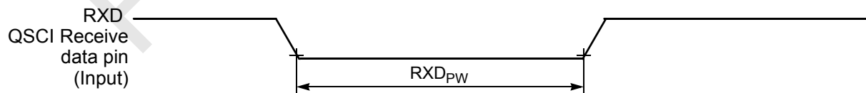
Figure 10-12 RXD Pulse Width
