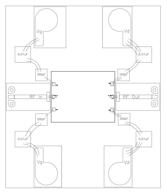
Note: Apply bias for Vd on both sides. Bias may be applied for Vg from either side.
