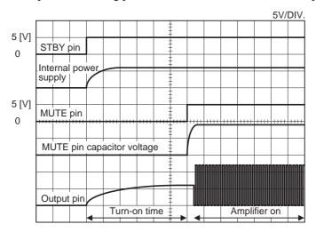
Turn-on time: the time between the point the STBY pin is set high and the point the MUTE pin is set high.
