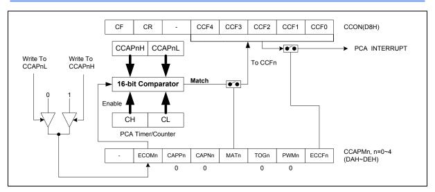
Figure 11-3 PCA 16-bit Timer Comparator Mode
