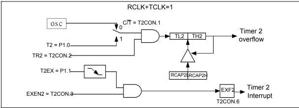
Figure 9-7 Baud Rate Generator Mode
