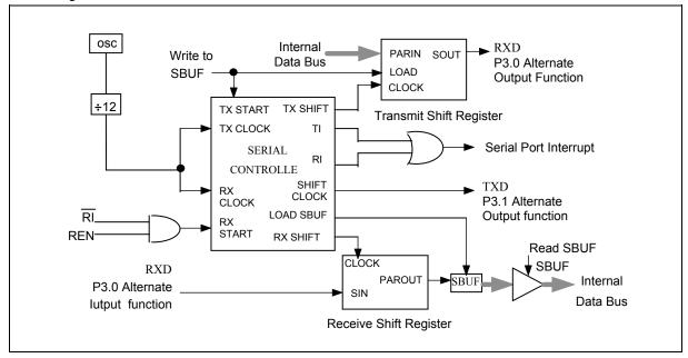
Figure 10-1 Serial Port Mode 0
