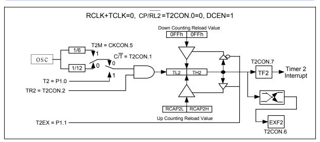
Figure 9-6 16-Bit Auto-reload Up/Down Counter
