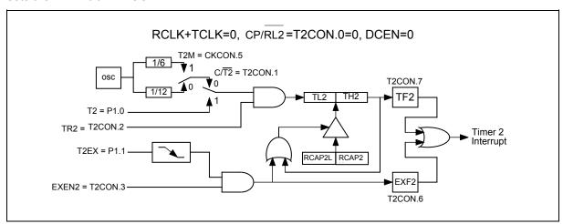
Figure 9-5 16-Bit Auto-reload Mode, Counting Up
