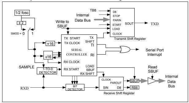
Figure 10-3 Serial Port Mode 2
