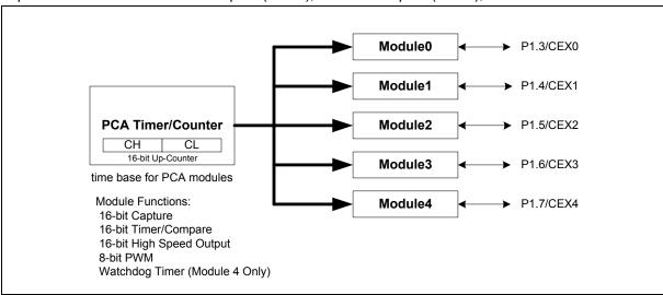
Figure 11-1 Programmable Counter Array (PCA)
