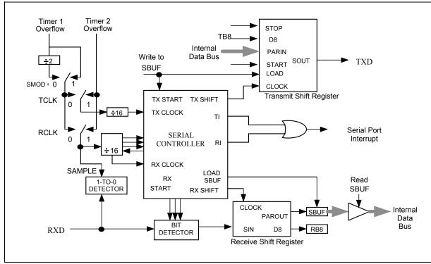
Figure 10-4 Serial Port Mode 3
