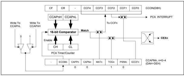
Figure 11-4 PCA High Speed Output Mode
