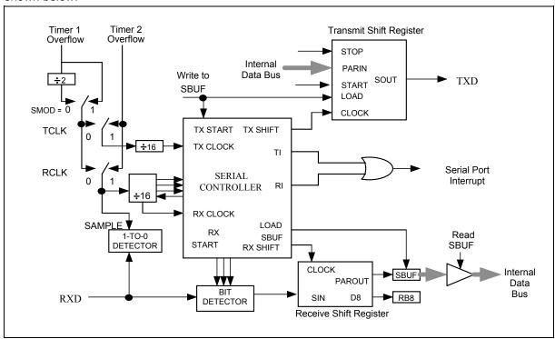
Figure 10-2 Serial Port Mode 1
