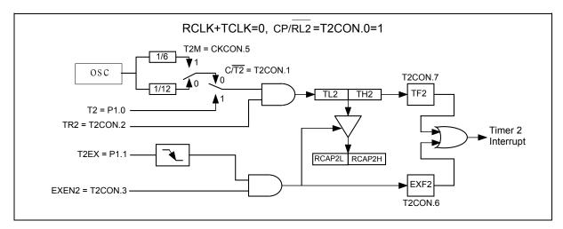
Figure 9-4 16-Bit Capture Mode
