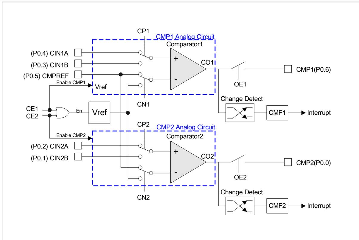
Figure 19-1: Analog Comparators
