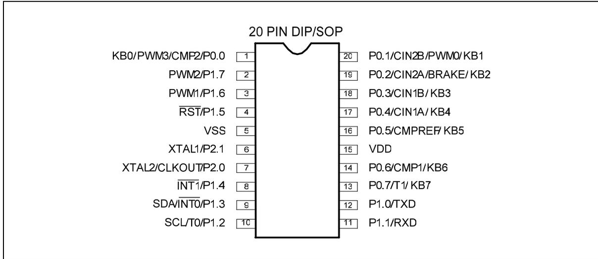
Figure 4-1: Pin Configuration
