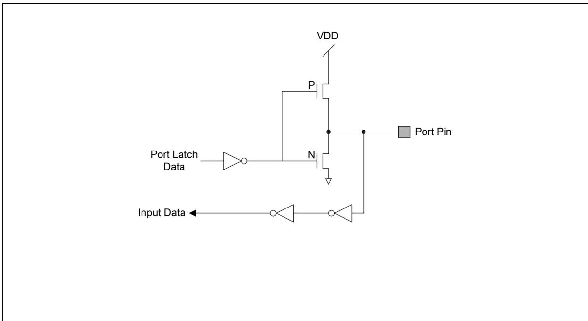
Figure 20-4: Push-Pull Output
