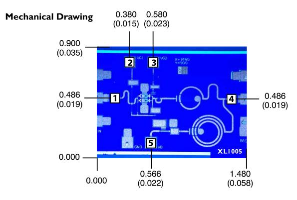
Units: millimeters (inches) Bond pad dimensions are shown to center of bond pad. Thickness: 0.110 +/- 0.010 (0.0043 +/- 0.0004), Backside is ground, Bond Pad/Backside Metallization: Gold All Bond Pads are 0.100 x 0.100 (0.004 x 0.004).
