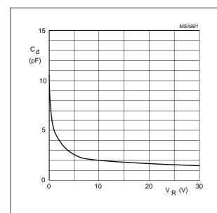
$f = 1 \text{ MHz}; T_{amb} = 25 \,^{\circ}\text{C}.$
