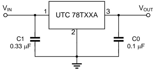
Note 1: To specify an output voltage, substitute voltage value for "XX".
