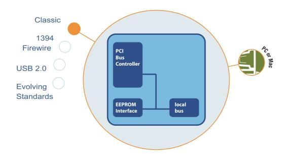
**The Oxford 9160 and 9162** deliver 8 and 32 bit local bus bridging in a simple and easy to implement solution. The generic bus supports Intel and Motorola modes with I/O or memory mapped configurations.
