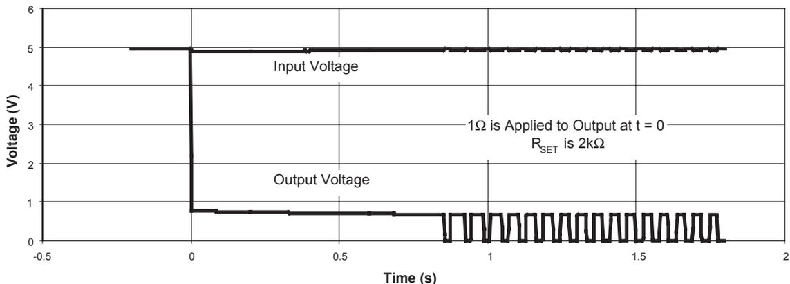
**Figure 1: Overload Operation.**
