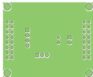
**Figure 3: AAT4601 Evaluation Board Solder Side Layout.**
