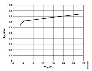
Figure 4. Supply Current vs. Supply Voltage
