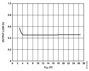
Figure 14. ALERT Output Low Voltage vs. Supply @ 1 mA
