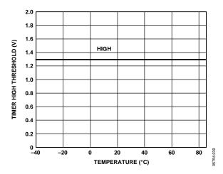
Figure 17. Timer Threshold vs. Temperature
