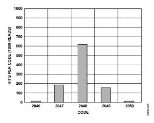
Figure 7. ADC Noise, Current Channel, Midcode Input, 1000 Reads
