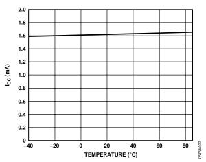
Figure 5. Supply Current vs. Temperature
