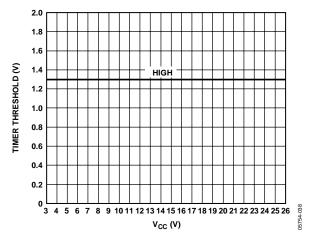
Figure 16. Timer Threshold vs. Supply Voltage
