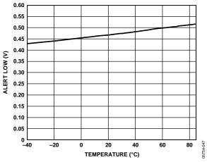
Figure 13. ALERT Output Low Voltage vs. Temperature @ 1 mA
