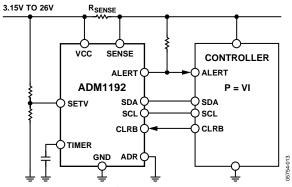
Figure 27. Using the ALERT Output as an Interrupt
