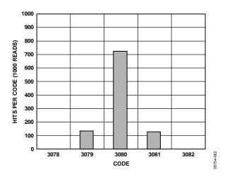
Figure 9. ADC Noise, 7:1 Voltage Channel, 5 V Input, 1000 Reads
