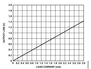
Figure 15. ALERT Output Low Voltage vs. Load Current
