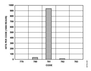
Figure 8. ADC Noise, 14:1 Voltage Channel, 5 V Input, 1000 Reads
