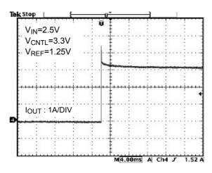
Fig. 7 Output Short-Circuit Protection (Sourcing)
