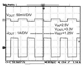
Fig. 8 Transient Response at 1.25V<sub>TT</sub>/1.5A
