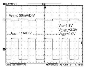
Fig. 9 Transient Response at 0.9V<sub>TT</sub>/1.5A
