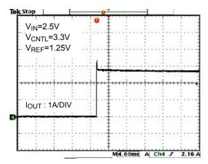
Fig. 6 Output Short-Circuit (Sinking)
