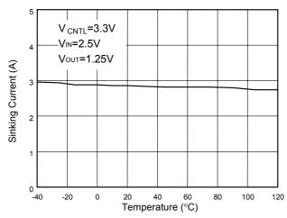
Fig. 5 Current-Limit (Sinking) vs. Temperature
