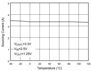
Fig. 4 Current-Limit (Sourcing) vs. Temperature
