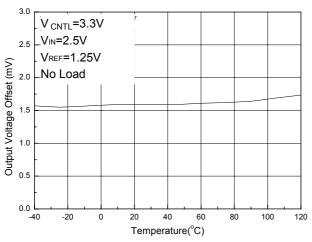
Fig. 3 Output Voltage Offset vs. Temperature
