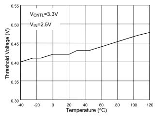
Fig. 1 Turn-On Threshold vs. Temp.
