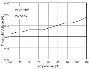
Fig. 2 Turn-On Threshold vs. Temp
