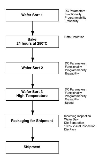
Figure 1. AMD KGD Product Test Flow
