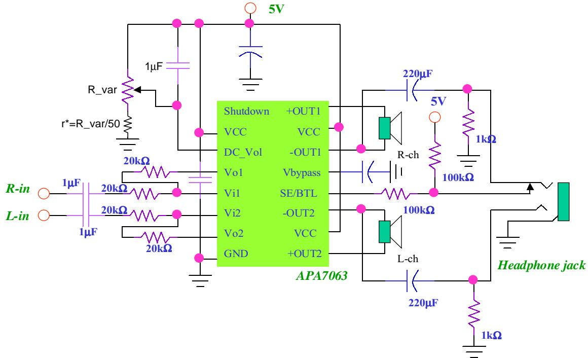
\* Add a resistor to avoid volume control gain error at power on status. For the R\_var with 10KΩ variable resistor, the recommended value of r is in range of 100~200Ω.
