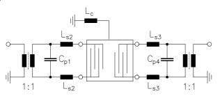
$$\begin{array}{ll} L_c &= 82 \text{ nH} \mid\mid 1.8 \text{ pF} \\ C_{p1} &= C_{p4} = 2.2 \text{ pF} \\ L_{s2} &= L_{s3} = 39 \text{ nH} \end{array}$$
