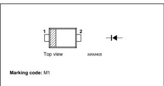
Fig.1 Simplified outline (SOD723A) and symbol.
