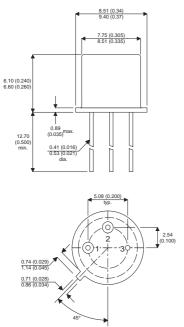
Bipolar NPN Device in a Hermetically sealed TO39 Metal Package.
