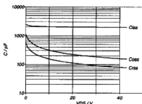
Fig. 12. Typical capacitances,  $C_{iss}$ ,  $C_{oss}$ ,  $C_{res}$ .
