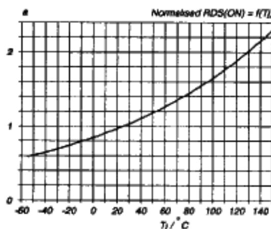
Fig. 9. Normalised drain-source on-state resistance.
