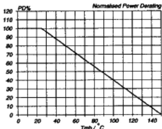
Fig.1. Normalised power dissipation.
