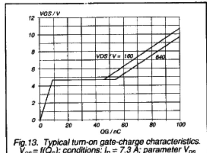
Fig.13. Typical turn-on gate-charge characteristics.
