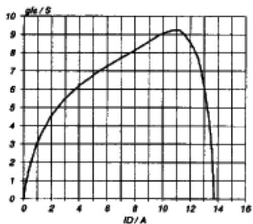
Fig. 8. Typical transconductance,  $T_J = 25^\circ C$ .
