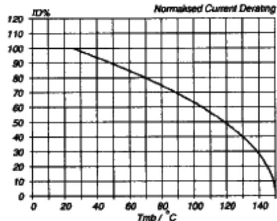
Fig.2. Normalised continuous drain current.
