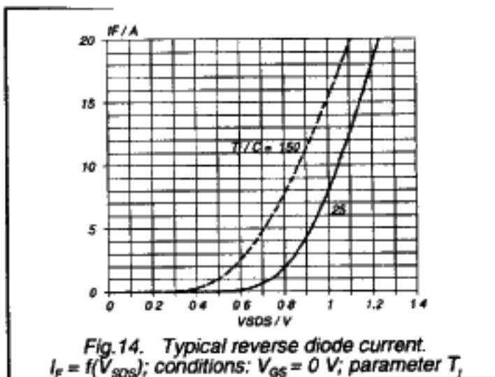
Fig.14. Typical reverse diode current.
