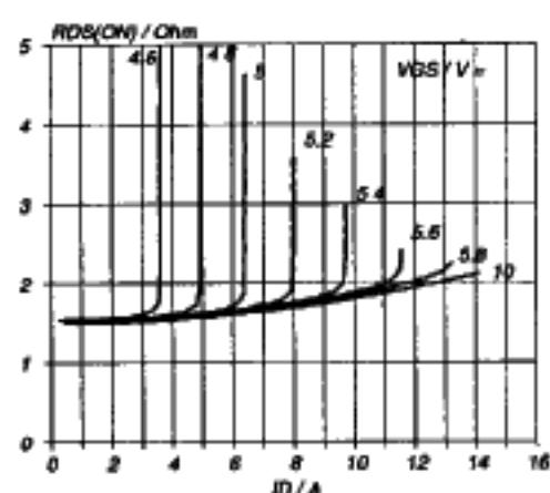
Fig.6. Typical on-state resistance,  $T_j = 25^\circ\text{C}$ .
