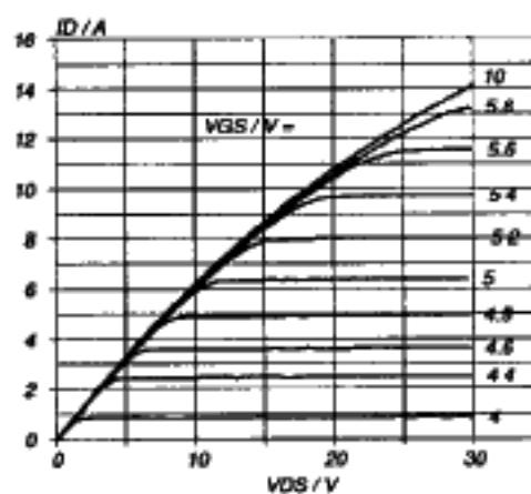
Fig.5. Typical output characteristics,  $T_j = 25^\circ\text{C}$ .
