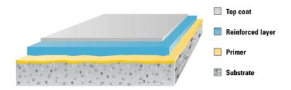
RINOL*LINING CR 543* is a chemical resistant lining system for steel and concrete substrates based on glass fibre reinforced vinyl ester resin.
