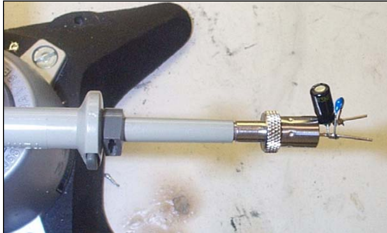
Figure 9 – Oscilloscope Probe with Probe Master 5125BA BNC Adapter. (Modified with wires for probe ground for ripple measurement, and two parallel decoupling capacitors added.)
