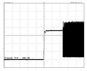
Figure 14 – 265 VAC Input and Maximum Load.  $V_{\text{DRAIN}},\,100$  V & 50 ms / div.
