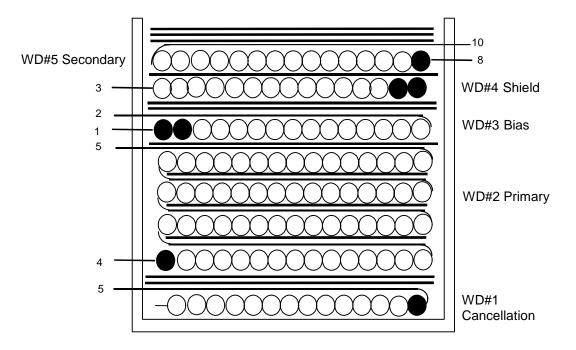
Figure 5 – Transformer Build Diagram
