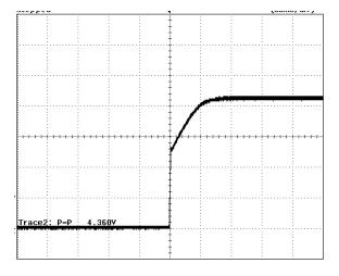
Figure 12 – Start-up Profile, 265 VAC 1 V, 50 ms / div.
