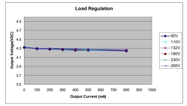
Figure 8 – Load Regulation, Room Temperature
