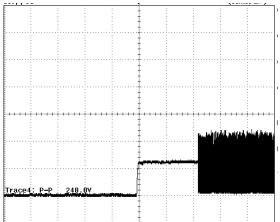
Figure 13 – 90 VAC Input and Maximum Load.  $V_{\text{DRAIN}},\,100$  V & 50 ms / div.
