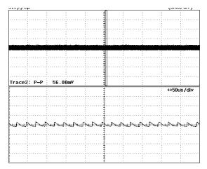
**Figure 18** – 5 V Ripple, 115 VAC, Full Load. 5 ms, 100 mV / div
