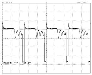
Figure 10 – 265 VAC, Full Load  $$V_{\text{DRAIN}}$, 100$  V, 10  $\mu\text{s}$  / div
