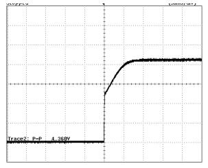
Figure 11 – Start-up Profile, 90VAC 1 V, 50 ms / div.
