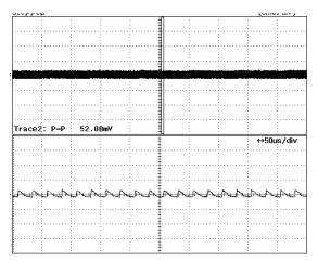
Figure 17 – Ripple, 90 VAC, Full Load. 5 ms, 100 mV / div
