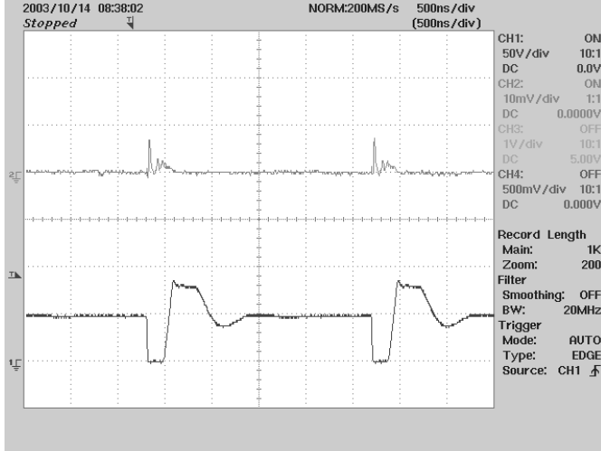
Figure 8 – 48 VDC, No Load. Upper: I_{DRAIN} , 1 A/div Lower: V_{DRAIN} , 50 V/div, 0.5 \mu s / div
