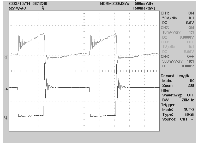
Figure 11 – 60 VDC Input, Full Load. Upper: I_{DRAIN} , 1 A/div Lower: V_{DRAIN} , 50 V/div, 0.5 \mu s / div
