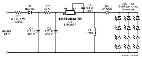
Figure 1. A 0.5 W, 12.9 V, 40 mA Constant Current LED Driver, Using a Non-Isolated Buck-Boost Topology.
