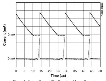
Figure 3. Output Current (Top Trace) and Input Current (Bottom Trace), 50 mA/div, 5 µs/div.
