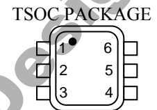
TOP VIEW 3.7mm x 4.0mm x 1.5mm
